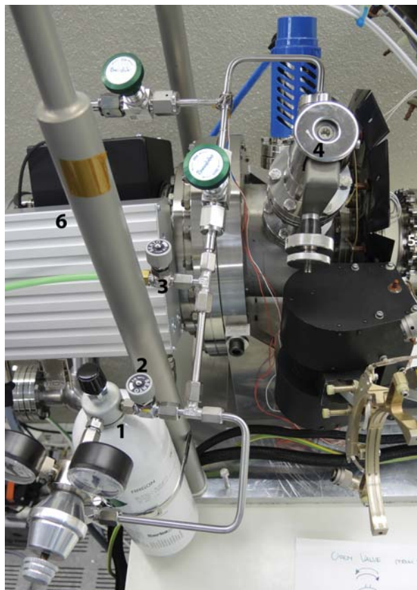
Fig. 2.1.4: Gas inlet: valve to bottle no. 1, bypass valve no. 2, valve to membran pump no. 3, leak valve no. 4, DFMS no. 5, turbo molecular pump no. 6.
