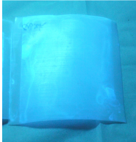
Figure D.5: Photograph of a Teflon sample coated with the pure solution. During the UVO treatment, the Teflon sample was fixated at two edges with tape onto the UVO treatment device. Below the tape the sample was not UVO treated, and therefore, the solution could not wet the sample along these edges.
