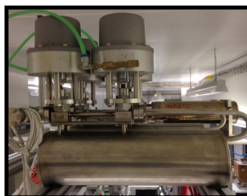
Figure 5.7: (a) Schematic viewing of the combination calibration gas bottle and pipette combination. (b) Picture of a calibration bottles in the lab.
