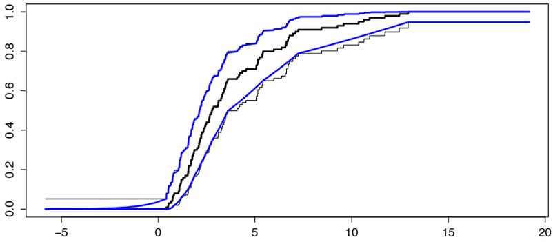
Figure 1.21.: Owen's band for  $F$  having concave  $\log F$  (Gamma distribution).
