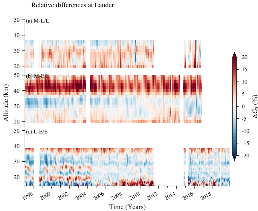
Figure 2. Relative ozone differences between (a) MWR (M) and lidar (L) data, (b) MWR and ERA5 (E) data, and (c) lidar and ERA5 data. Lidar and ERA5 profiles in (a) and (b) have been convolved with MWR averaging kernels.
