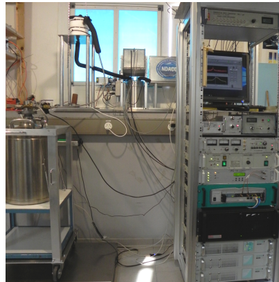
Figure 4.2: The GROMOS radiometer in a temperature-controlled room at the University of Bern.
