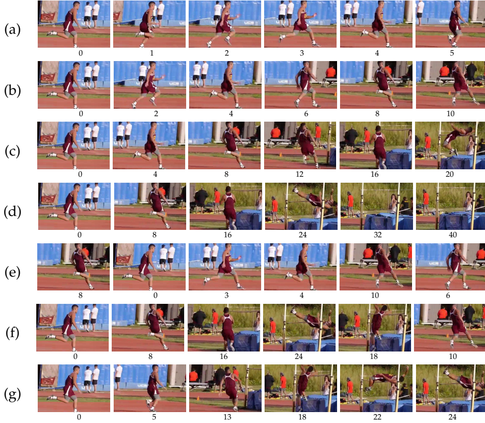
FIGURE 5.1: Learning from temporal transformations. The frame number is indicated below each image. (a)-(d) speed : skip 0 frames (a), 1 frame (b), 3 frames (c), or 7 frames (d). (e) random : frame permutation. (f) periodic : forward-backward motion (at the selected speed). (g) warp : variable frame skipping while preserving the order.
