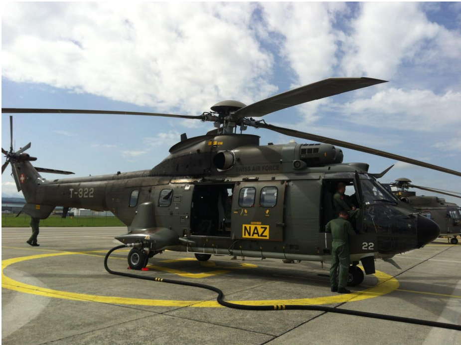
Fig. 18: Helicopter equipped with 4 detectors for airborne gamma ray spectrometry.
