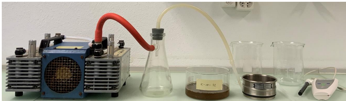
Figure S1.5: Laboratory equipment required for aspiration and rinsing of fPOM from bulk soil.
