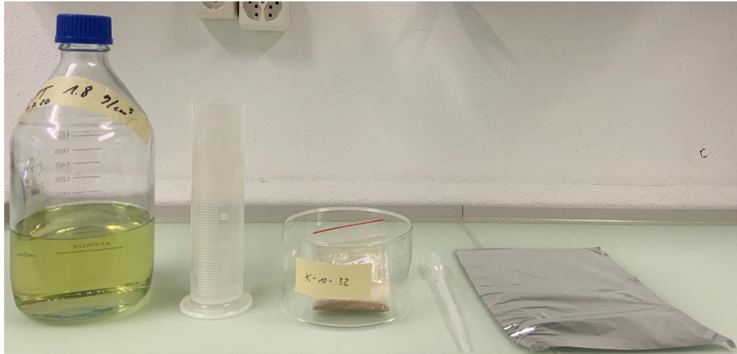
Figure S1.3: Laboratory equipment required for adding density solution to soil samples.
