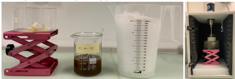
Figure S1.7: Laboratory equipment required for ultrasonication of the mineral soil.
