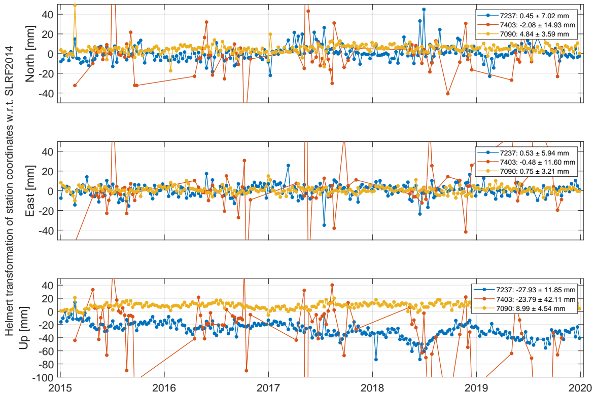
Figure 6.17: Time series of the Helmert transformation from the estimated station coordinates w.r.t. SLRF2014 in North, East and Up for the SLR stations 7237 (blue), 7403 (orange) and 7090 (yellow) for the years 2015-2020. The datum definition is realized by using the ILRS core station list without the Helmert approach.
