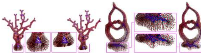
Figure 3.25: Dpoints representations under different shape priors. When there are C^1 discontinuities between known and missing surfaces, using the volume preserving shape prior (left) results in “blobby” shapes. The minimal volume shape prior can be applied to alleviate this problem (right).
