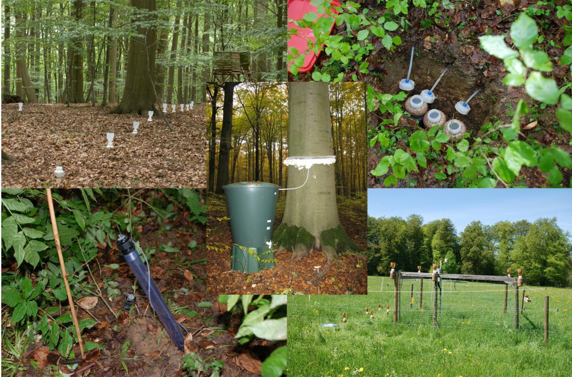
**Figure 1.6:** Sampling devices for forest throughfall (top left), litter leachate (top right), stemflow (center), arrangement of rainfall and throughfall samplers in grasslands (bottom right), and mineral soil solution (bottom left). The center picture was provided by Sebastian Bischoff.
